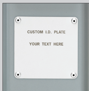
ID PLATE (Type H, Style IV) Per MIL-P-15024 Size 10 4" x 4" x .020" (102x102x0.5 mm), aluminum fastener attached.
