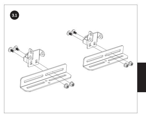
ASSEMBLE TWO PINNED BRACKET ASSEMBLIES AS SHOWN, USING M6 CARRIAGE BOLTS AND LOCKNUTS. ONLY PARTIALLY TIGHTEN NUTS TO ALLOW FINAL ADJUSTMENT WITH CASE POSITION.
