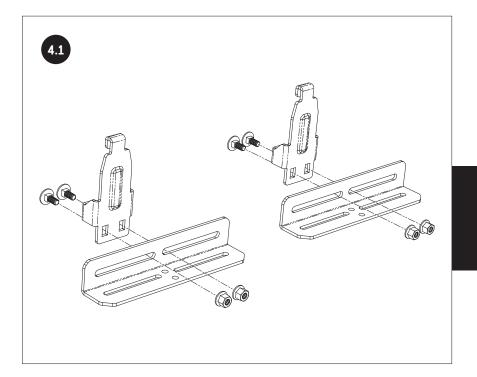
ASSEMBLE TWO FIXED BRACKET ASSEMBLIES AS SHOWN, USING M6 CARRIAGE BOLTS AND LOCKNUTS. ONLY PARTIALLY TIGHTEN NUTS TO ALLOW FINAL ADJUSTMENT WITH CASE POSITION.
