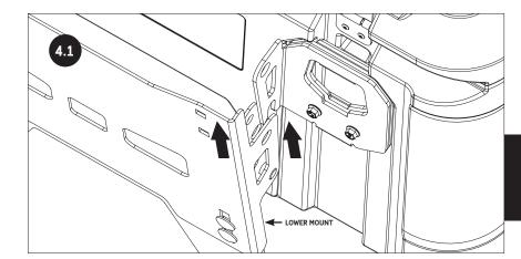
SLIDE LOWER MOUNT UP TO ENGAGE FIXED BOTTOM PINS IN EARHOOKS ON CASE CLAMPS.
