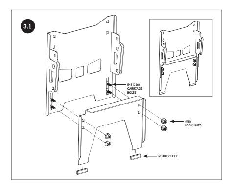
FIT FOUR (M8 X 16) CARRIAGE BOLTS THROUGH SLOTS IN LOWER MOUNT TO ASSEMBLE FOOT PLATE WITH (M8) LOCK NUTS.
