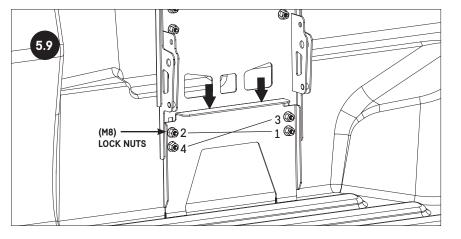
TIGHTEN FOUR (M8) LOCK NUTS ON FOOT PLATE WHILE PUSHING DOWNWARDS TO MAINTAIN GOOD FOOTING.
