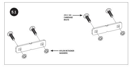
ASSEMBLE FOUR (M8 X 30) CARRIAGE BOLTS THROUGH SLOTS IN NUT PLATES TO NYLON RETAINER WASHERS.
