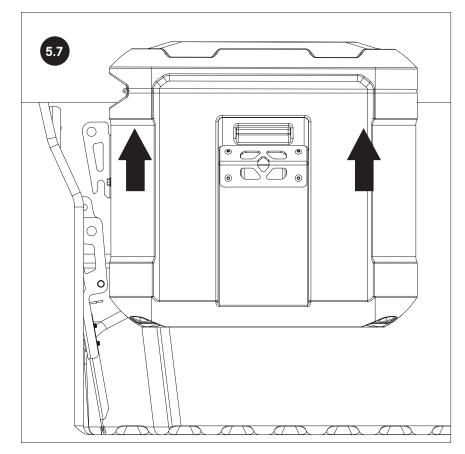
REMOVE TWO CLEVIS PINS AND LIFT CASE UP AND OUT OF WAY TO ALLOW ACCESS TO FOOT PLATE FOR FINAL ADJUSTMENT.
