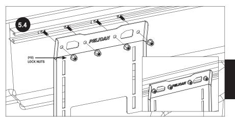
FIT UPPER MOUNT TO STUD PLATE ASSEMBLIES USING 4 (M8) LOCK NUTS.
