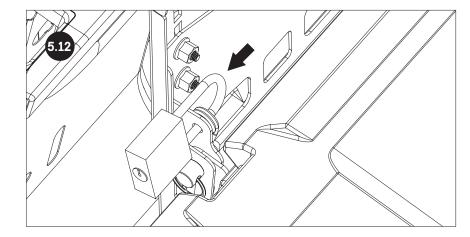
FOR THEFT DETERRENCE, SECURE R-CLIP TO TRUNK CLAMP WITH PADLOCK (NOT INCLUDED) ON ONE OR BOTH SIDES OF TRUNK AS SHOWN.
