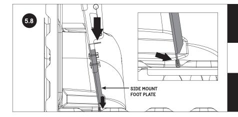
PUSH DOWN FIRMLY ON FOOT PLATE TAB TO SEAT FOOT INTO BED FLOOR, FOOT MUST CATCH ON EDGE OF BED RIB AS SHOWN.
