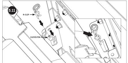
INSERT BOTH CLEVIS PINS SO THAT CLIP HOLES ARE INSIDE MOUNTING EARS AND FACING UPWARD.
