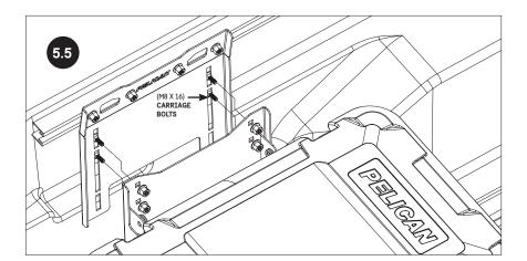
WITH LOWER MOUNT PINNED TO THE CASE, PLACE ASSEMBLY INTO TRUCK BED. ALIGN UPPER AND LOWER MOUNTING PLATES.
