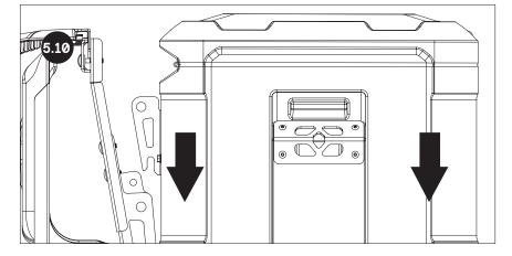
RE-INSTALL TRUNK BY LIFTING IT AND LOWERING CLAMP HOOKS ON TO THE LOWER MOUNT PINS.
