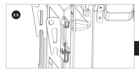
CLAMP SHOULD BE SECURE AGAINST SLIDING OR ROTATION, WITH MOUNTING EAR VERTICAL.
