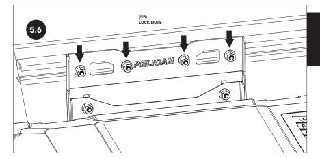
IMPORTANT: CLEVIS PINS ARE TO BE KEPT IN PLACE FOR THIS NEXT TIGHTENING STEP:
