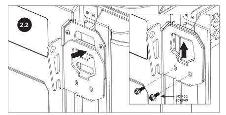
SLIDE CLAMP UPWARDS WITH HOOKS INSERTED IN TOP SLOT AND ON BOTTOM EDGE OF TIEDOWN PLATE.
