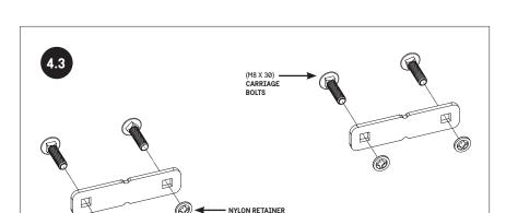
ASSEMBLE FOUR (M8 X 30) CARRIAGE BOLTS THROUGH SLOTS IN NUT PLATES TO NYLON RETAINER WASHERS.
