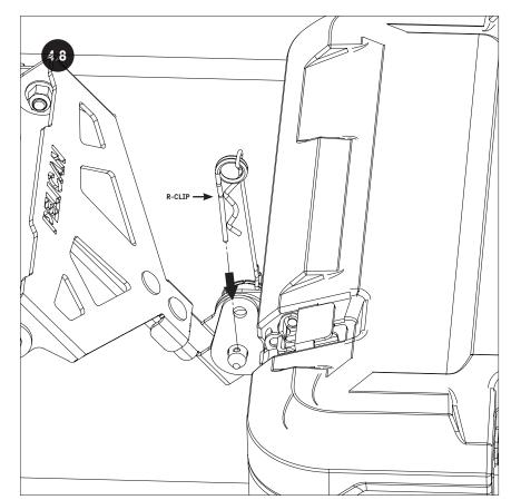
INSERT R-CLIP AS SHOWN TO SECURE CLEVIS PIN.
