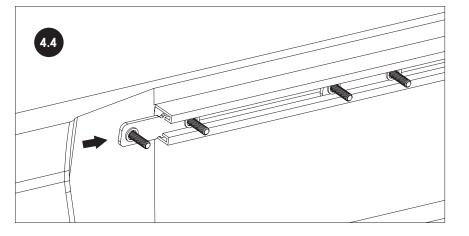
SLIDE PAIR OF NUT PLATE ASSEMBLIES INTO BED RAIL.
