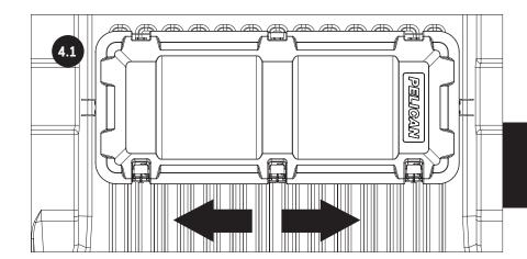
PLACE CASE IN DESIRED TRUCK BED LOCATION TO DETERMINE LOCATION OF MOUNTING BRACKETS.
