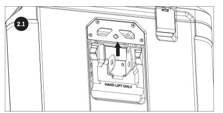
INSTALL CASE PLATE CLAMP TO TIEDOWN PLATE.
