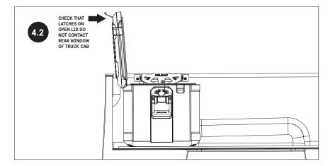
ENSURE ADEQUATE CLEARANCE FOR LID OPENING. CHECK THAT LATCHES ON OPEN LID DO NOT CONTACT REAR WINDOW OF TRUCK CAB.
