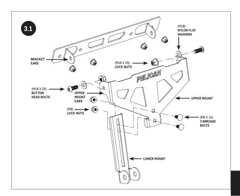
ASSEMBLE UPPER AND LOWER MOUNTS TO BRACKETS
