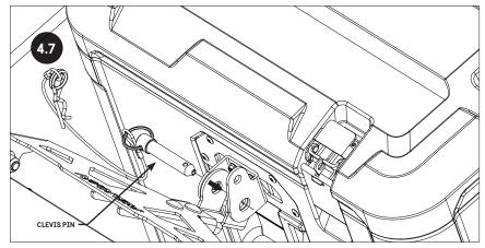
SWING MOUNT UPWARDS BETWEEN CASE CLAMP EARS, AND ADJUST LOWER MOUNT LENGTH TO INSERT CLEVIS PIN THROUGH BOTH PARTS.
