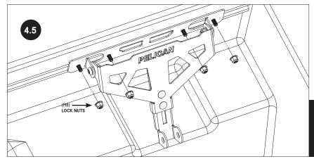
POSITION NUT PLATES TO LINE UP WITH MOUNT ASSEMBLY AND FIT FOUR (M8) LOCK-NUTS. PARTIALLY TIGHTEN NUTS TO ALLOW SLIDING ADJUSTMENT WITH CASE POSITION AND OPPOSITE MOUNT ASSEMBLY.
