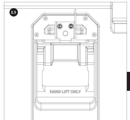
CLAMP SHOULD BE SECURE AGAINST SLIDING OR ROTATION, WITH MOUNTING EARS VERTICAL.
