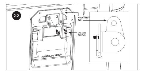
CENTER CLAMP LEFT TO RIGHT TO ALIGN SCREW HOLES WITH PLATE SLOTS.
