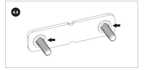
SLIDE NYLON RETAINER WASHERS FIRMLY AGAINST NUT PLATES TO TIGHTLY SEAT SQUARE BOLT FEATURES IN SLOTS AS SHOWN.
