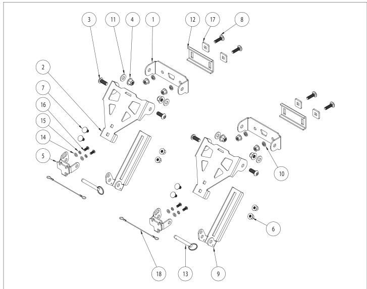
SLIDE PLATE CLAMP UPWARDS WITH U-BEND ENCLOSING CASE PLATE.
