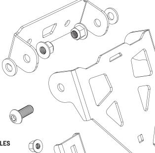
FIT TWO (M8 X 16) CARRIAGE BOLTS IN SQUARE HOLES FROM FRONT OF UPPER MOUNT THROUGH SLOT IN LOWER MOUNT. FASTEN (M8) LOCK NUTS LOOSELY TO ALLOW ADJUSTMENT LATER.
