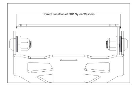
FASTEN (M10) LOCK-NUTS SNUGLY BUT ALLOWING ROTATION OF MOUNT.
