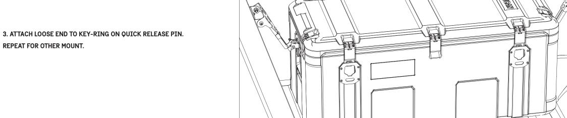
3. ATTACH LOOSE END TO KEY-RING ON QUICK RELEASE PIN.
