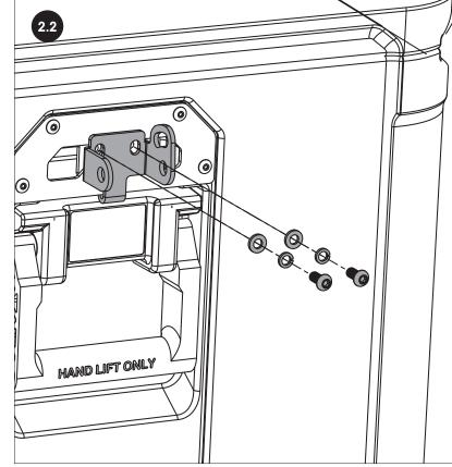
KEEP CLAMP VERTICAL AS SHOWN WHILE TIGHTENING SCREWS WITH M4 ALLEN TOOL TO SECURE FIRMLY IN PLACE.
