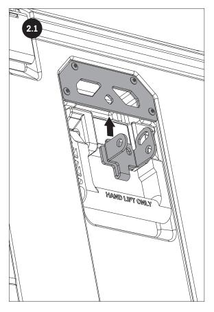
CENTER CLAMP LEFT TO RIGHT TO ALIGN SCREW HOLES WITH PLATE SLOTS.
