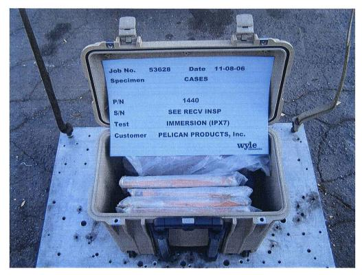
Photograph 3 Immersion Test Setup
